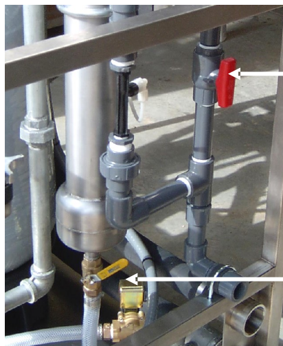
Ozone manifold injector bypass valve Adjust to obtain 5 LPM on ozone flow meter
