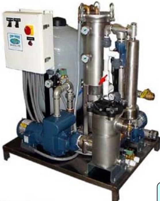
Self-Contained unit with 316 stainless steel self-cleaning filter and onboard ozone recirculation. Epoxy coated aluminum filter housings and stainless steel piping to prevent corrosion.
