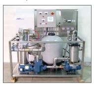
Systems incorporate bag filters or permanent stainless steel self-cleaning filters to provide high quality water at flow rates to 125 gallons per minute. Higher
